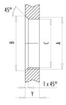
Installation direction: o-ring sits on chamfer.
